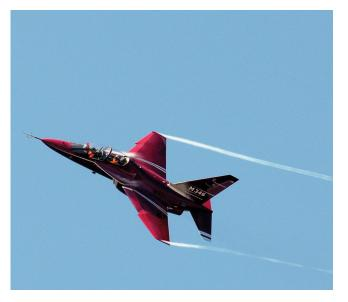
A military transonic trainer aircraft designed for training combat pilots for front line fighter aircraft, the Alenia Aermacchi M-346 Master is powered by a digital flight control system.
