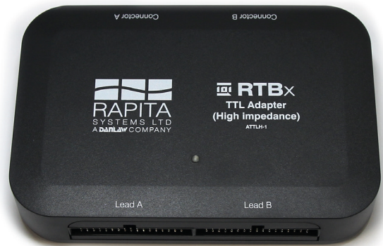
Figure 5. RTBx adapter (high impedance TTL)
