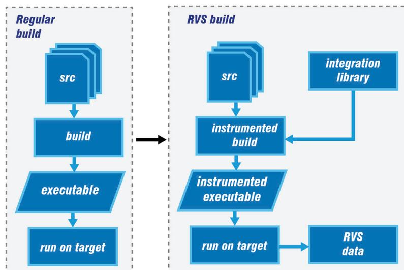
Figure 1: Integrating RVS into a development environment
